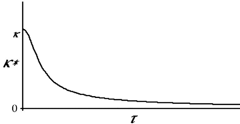
Figure 2. The effective thermal conductance \kappa^* as a function of the cycle time \tau . Note that as \tau tends to zero, \kappa^* approaches \kappa .
